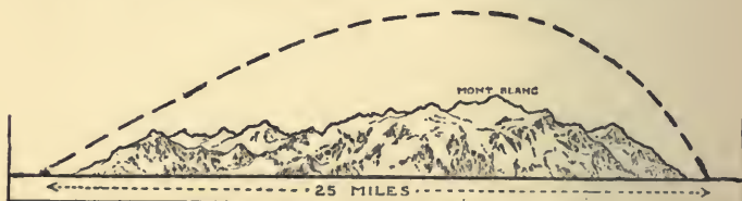
[Curve of flight, or trajectory, of 850 lb. projectile from a Dreadnought 12-in. turret-gun fired with full service charge.]
